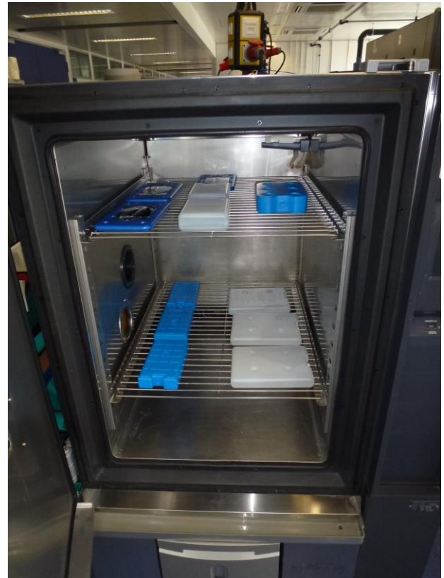
2. Conditioning of cooling packs at -18°C
