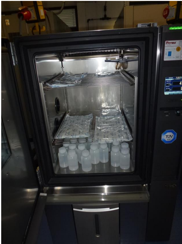
1. Conditioning of samples and thermal barriers at 4°C
